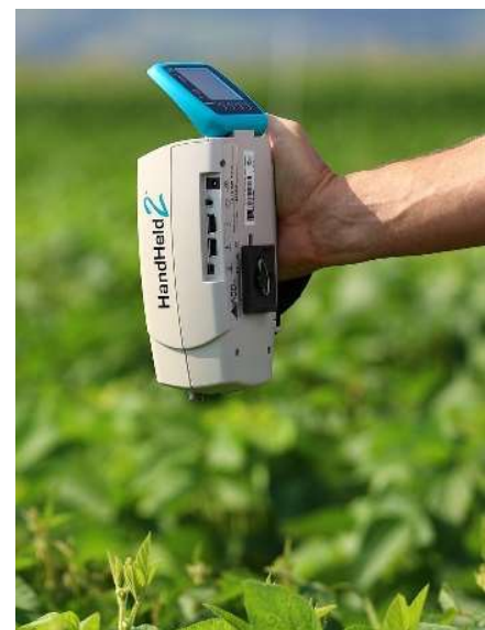
Fig. 2: Hyperspectral reflectance measurement of soybean breeding lines in the field with a handheld sensor. (Photo credits: J. Vollmann)
