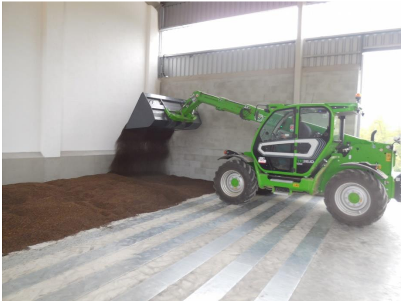
Fig. 2: Perforated floor active drying with ambient air at EKOFARMA PROBIO s.r.o. (URL: https://rb.gy/703v )
